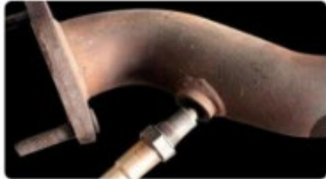
Second Step: Take off the old sensor spacer
