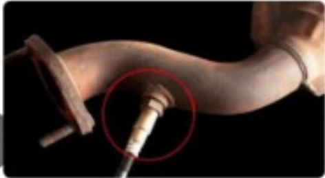
First step: Find the position for sensor spacers
