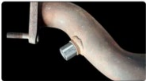
Third Step: Put on the new sensor spacer to the car
