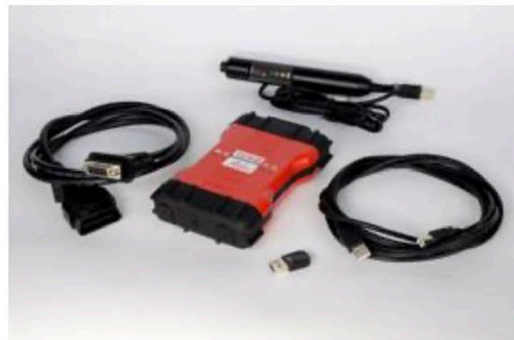
**VCM II** - The discontinued VCM II is a diagnostic hardware Vehicle Communication device. The VCM II is still capable of performing full dealership level diagnostics on 1996 to present Ford and Lincoln vehicles when used with Ford Diagnostic Software including IDS and FDRS. The VCMII was discontinued due to aging hardware components and
